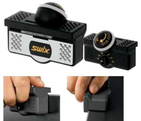
TA3002XF Adjustable file edge holder with 40 mm file. Side edge can be adjusted from 90° to 85°. Base edge from 0.5° to 1°.
